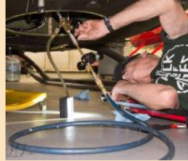
Steve with his pressure gauge metering system at work searching for possible leaks in the fuel system.
