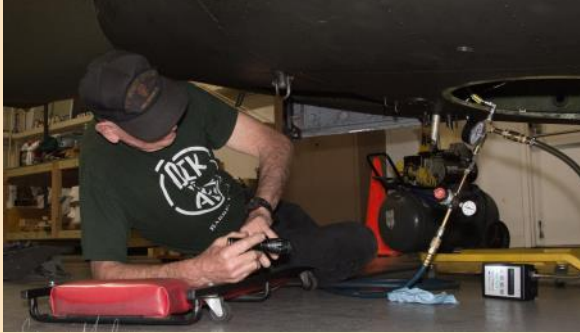
Steve with his pressure gauge metering system at work searching for possible leaks in the fuel system.
