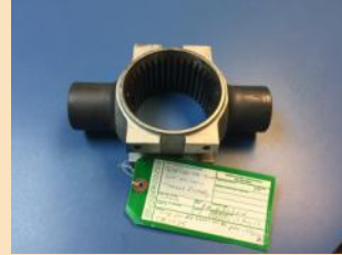
Part # 204-011-105-1. Trunnion. AD 200-01-31 requires that we replace this since we have not yet been able to establish Time In Service for the part.
