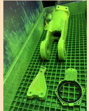
Parts of our main rotor head/hub assembly undergoing dye penetrant testing at East Coast Propellers in Lititz, PA. Randy and his team did a fantastic job for us on getting these crucial parts inspected.
